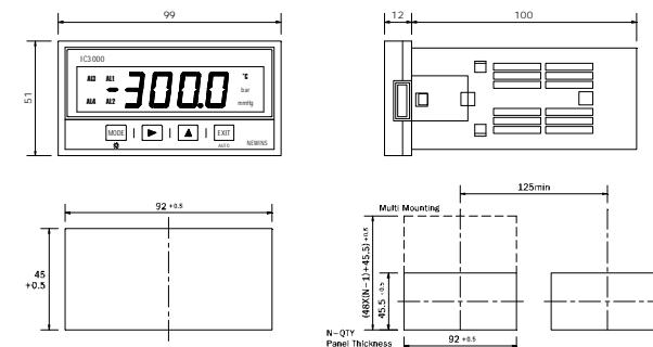
⚠ Caution : Maintenance and to ensure the safety of the device if you add a space to more than 125mm size is recommended.
