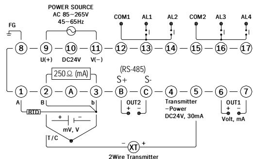
\* mA Input(+ -) Needs 250 OHM 0.05% 25ppm Resistance (2, 3 Pin)
